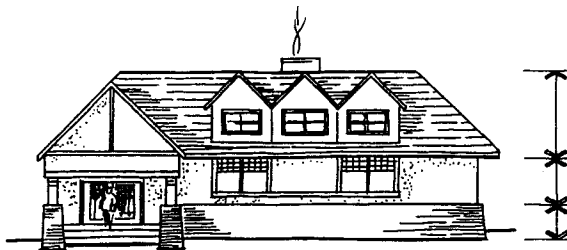
Fig. 3.39 Traditionally Jasper's housing had an identifiable base, middle and top. Second storey rooms were often built right into the roof.
