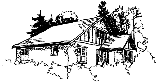
Fig. 2.5 Steep roofs with large overhangs are a traditional form
